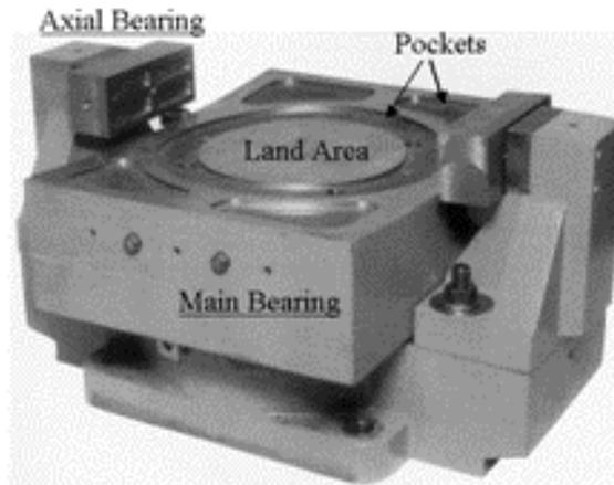
Figure 2.3-1. Typical Hydrostatic Bearing.
