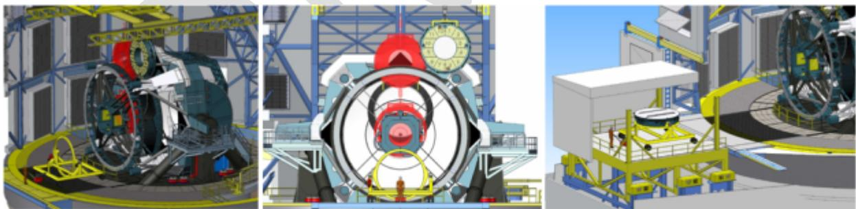
The SMA is Removed By the Dome Crane, then secured to the SMA Cart and Rotated
