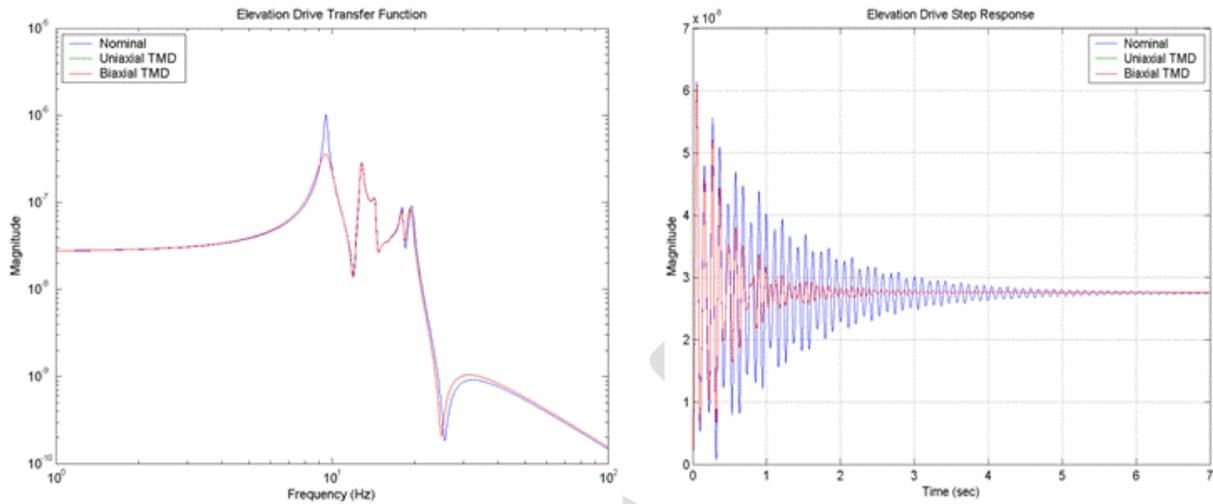
Fig.2.10-2 Effects of Added Damping on TMA Dynamic Performance.
