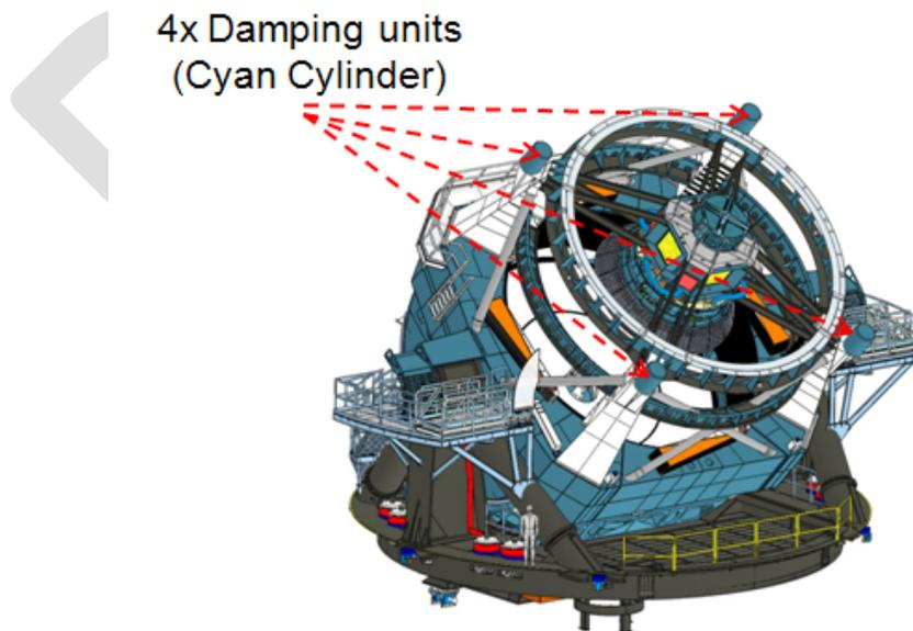
Fig.2.10-1 Location of damping units on telescope.
