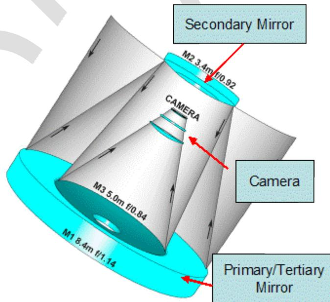
Figure 1.1-1. Optical Arrangement.
