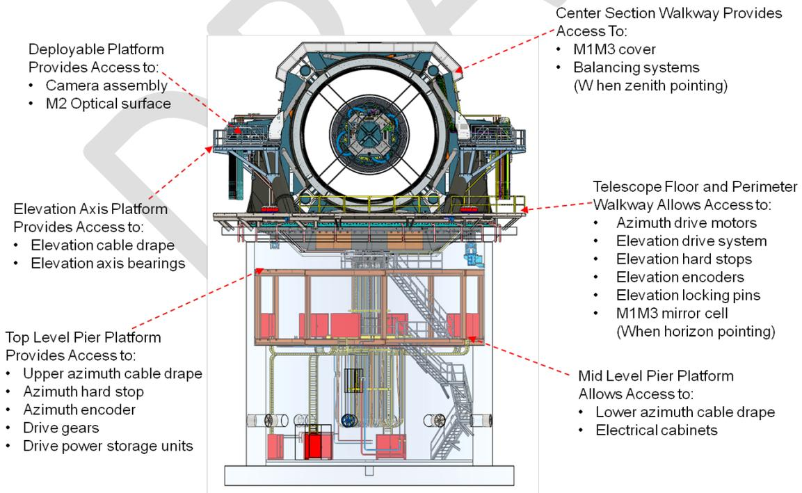
Figure 1.2-4. Platforms, Stairs and Ladders Provide Access to All Critical Components.
