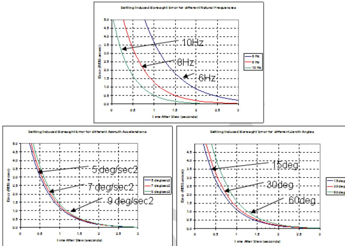
Figure 3.4-1: Settling time as a function of natural frequency, peak acceleration and zenith angle.
