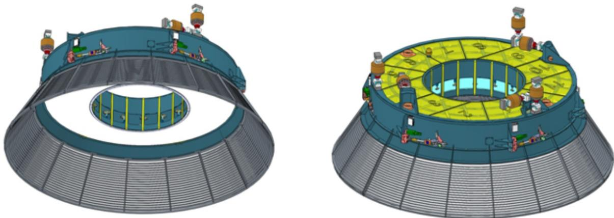
Fig 7.2-1: M2 Combined Assembly: Mirror Cell Assembly, Light Baffle, Hexapod.
