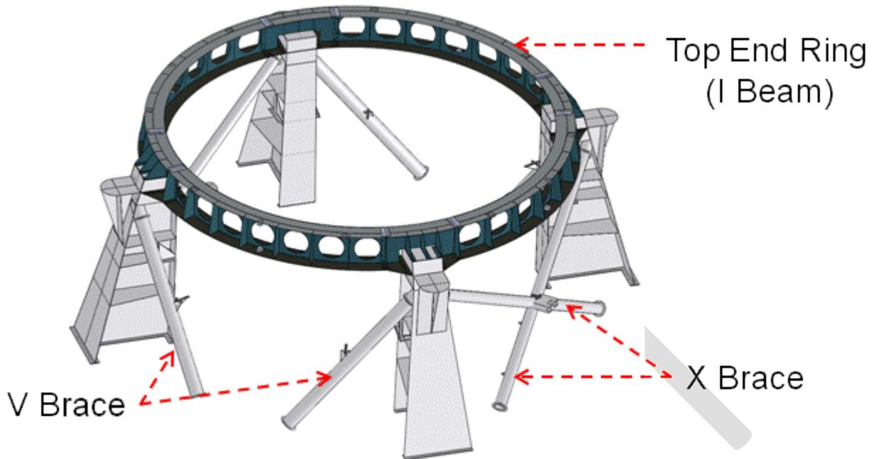
Figure 2.2.1-4. Top End Assembly Structure, TEA Ring, TEA Piers and TEA Braces.
