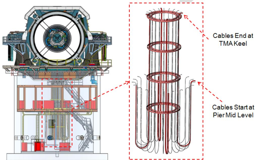
Fig. 2.6.1-1. Azimuth Cable Drape.
