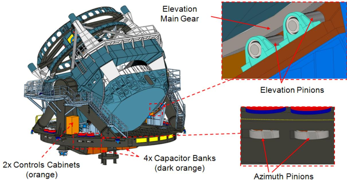
Fig. 2.4-1. Drive System Components
