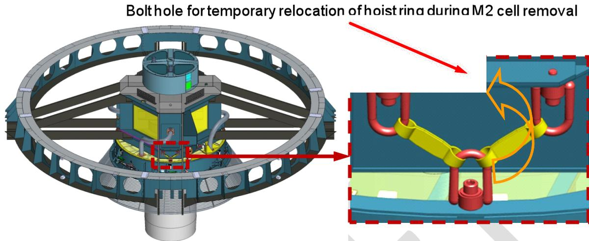
**Figure 7.2-4: M2 Mirror Cell Assembly Restraining Straps**
