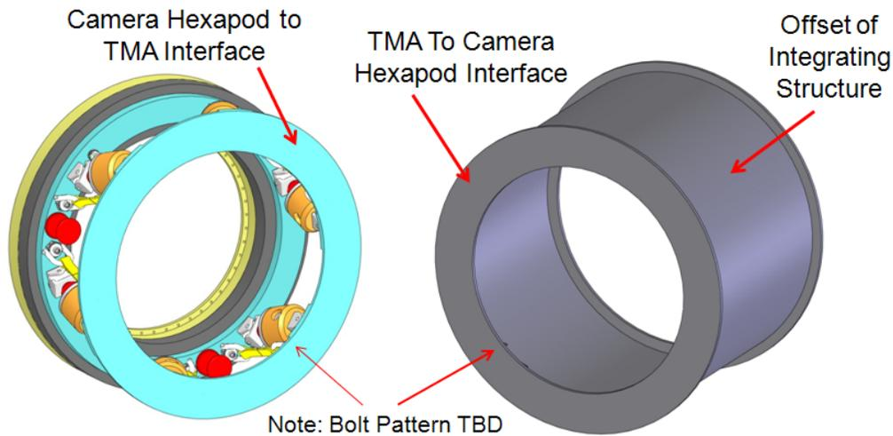
Figure 7.3.2-1: Camera Hexapod To Telescope Mount Assembly (TMA) Interface.
