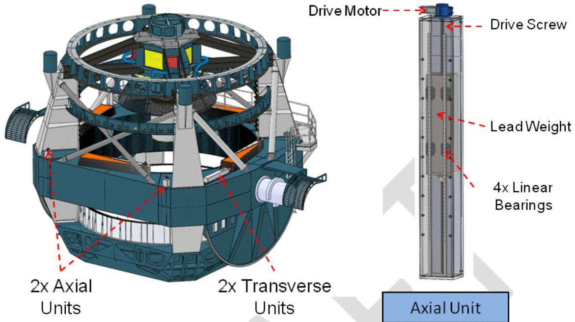
Fig.2.9-1 Elevation Assembly Balancing System.
