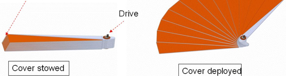
Fig.2.8-2. M1M3 Mirror Single Fan Assembly.
