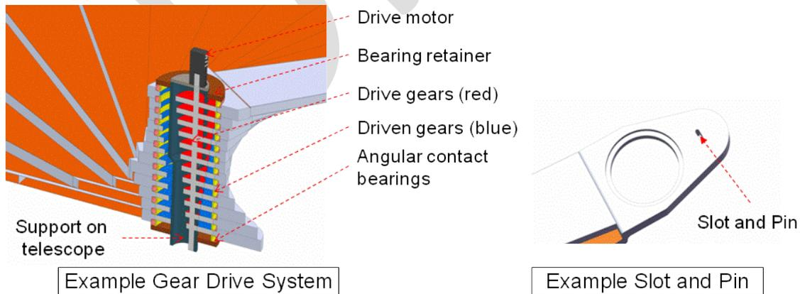
Fig.2.8-5 Drive System of M1M3 mirror cover.
