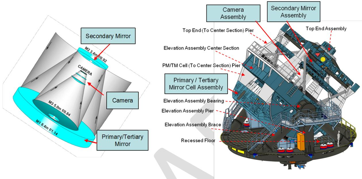
Figure 1.2-2. TMA Accommodation of Optical System.
