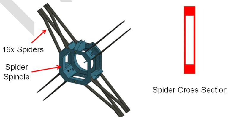
Figure 4-2: Spider Spindle and Spiders
