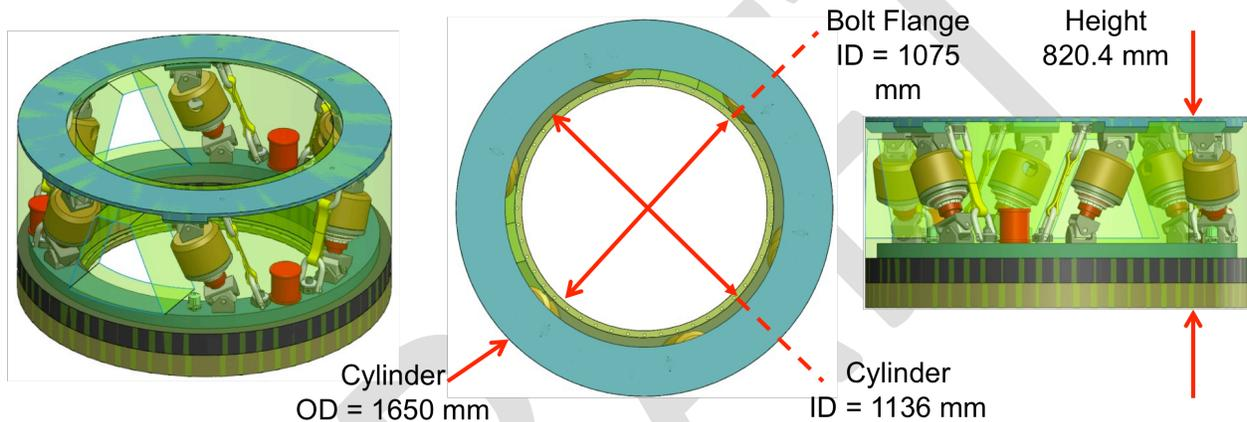
Figure 7.3.1-1: Design Envelope of Camera Hexapod/Rotator Assembly
