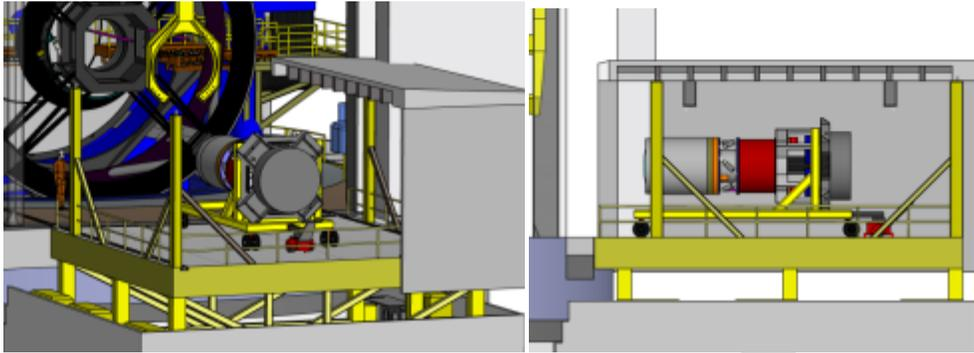
Figure 7.3.5-1: Camera Support Assembly on Cart.
