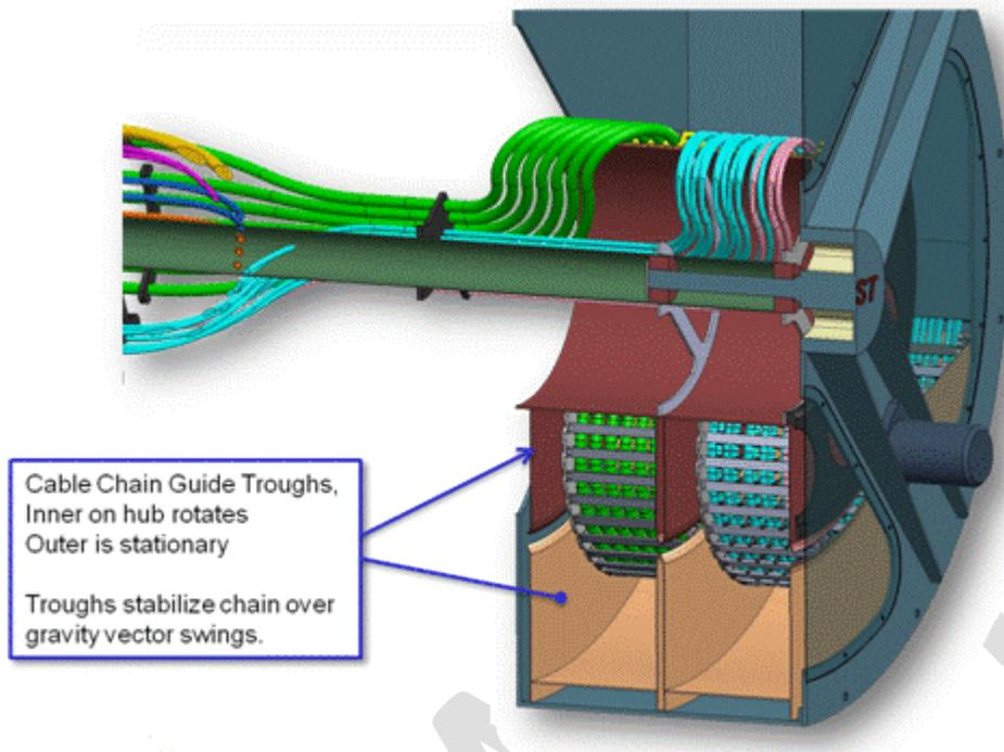
Fig. 2.6.3-2. Section View of Camera Cable Wrap.
