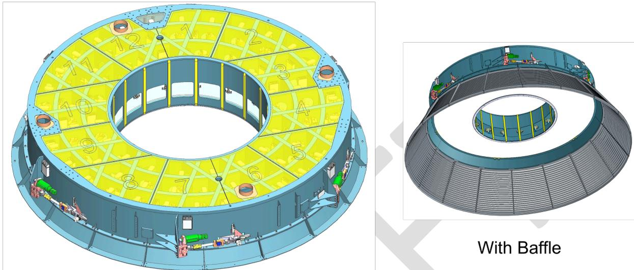
Figure 7.2-3: M2 Mirror Cell Assembly (With and Without Baffle)
