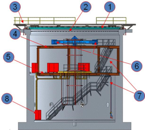
Figure 6-1: Components of telescope pier.
