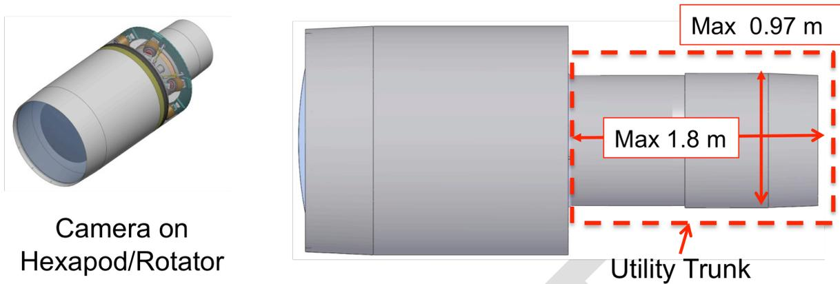
Figure 7.3.1-2: Design Envelope of Camera Hexapod/Rotator Assembly
