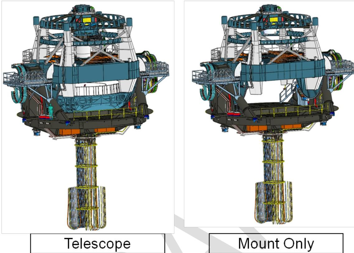
Figure 1.2-1. Telescope (Left) Vs. Telescope Mount Assemble (right).
