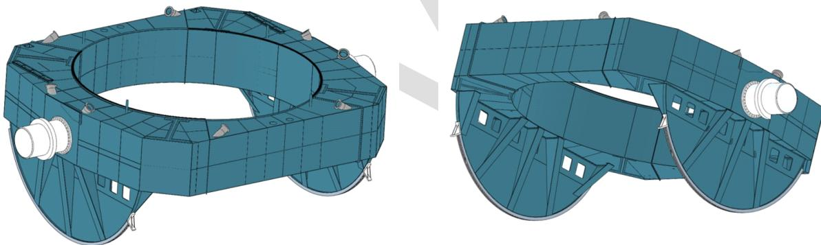
Figure 2.2.1-2. Center Section w Drive Wheels.
