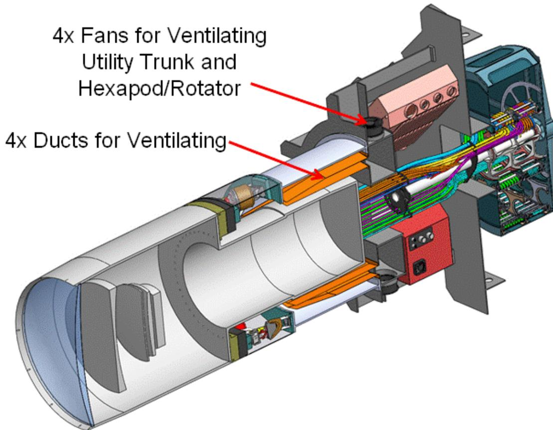
Figure 5.3-2: Thermal Control of Camera Hexapod/Rotator and Camera Utility Trunk.
