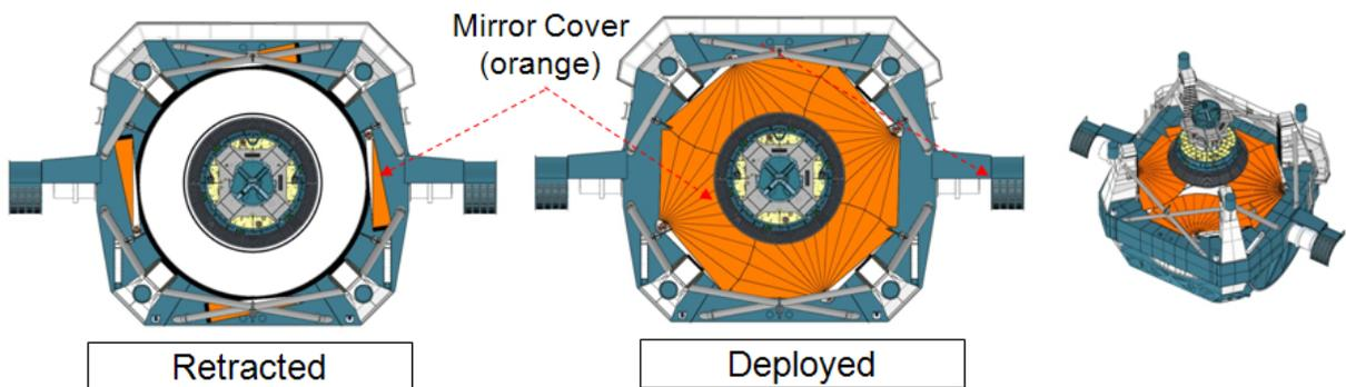
Fig. 2.8-1. M1M3 Mirror Cover shown on TMA elevation assembly
