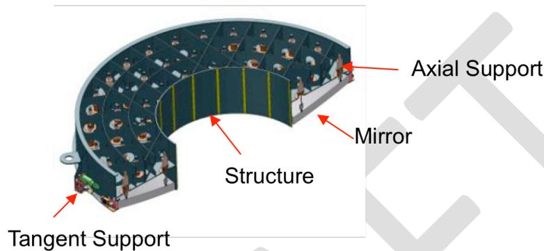
Figure 7.2-2: M2 Mirror Cell Assembly (cover panels and thermal control system not shown)
