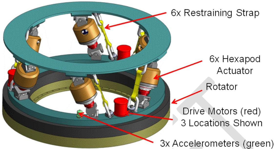
Figure 4.2.1-1: Camera Hexapod/Rotator Assembly
