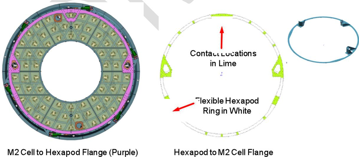
Figure 7.2.2-2: M2 Mirror Cell Assembly to M2 Hexapod Interface
