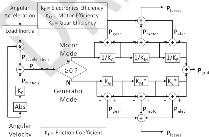
Figure 3.6-1: Schematic of Drive Power Scheme.
