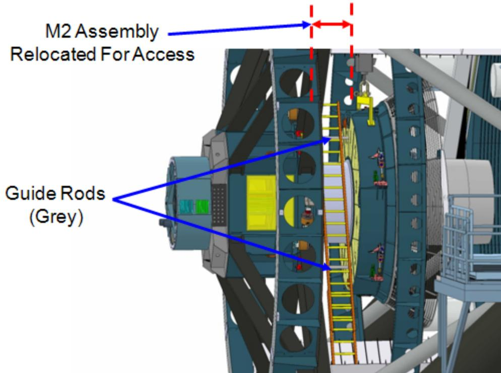
Figure 7.2.4-1: M2 Mirror Cell Assembly Special Access Configuration
