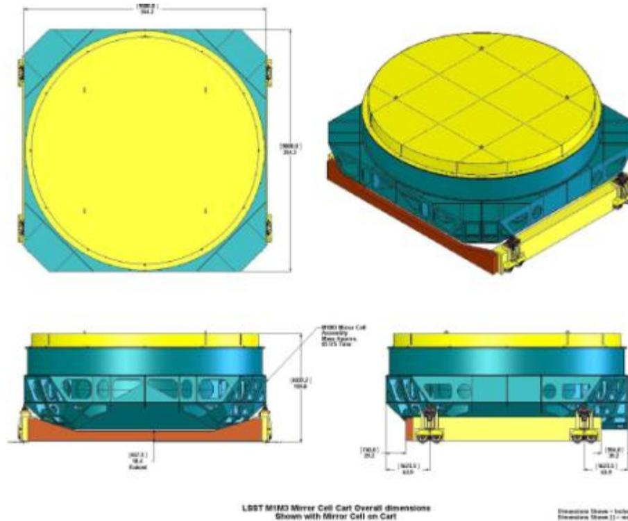
Fig. 7.1.4-1. M1M3 mirror cell assembly on cart.
