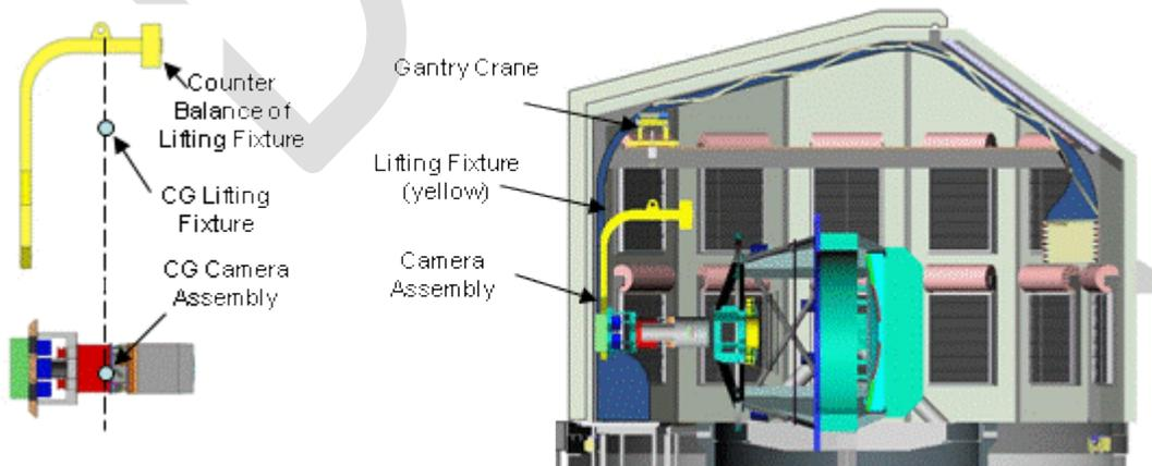
Fig. 4.1-2. Camera support assembly installation/removal
