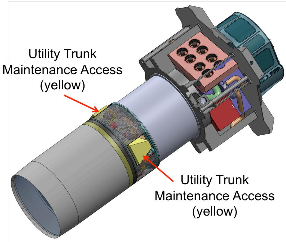
Figure 7.3.3-1: Maintenance Assess Between Actuator Actuators
