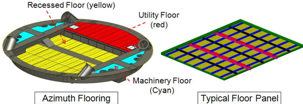
Fig.2.12.1-1 Main Floor of TMA Azimuth Assembly.
