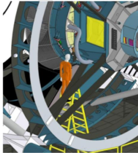
Figure 7.2.3-1: On Telescope Access to the M2 Combined Assembly
