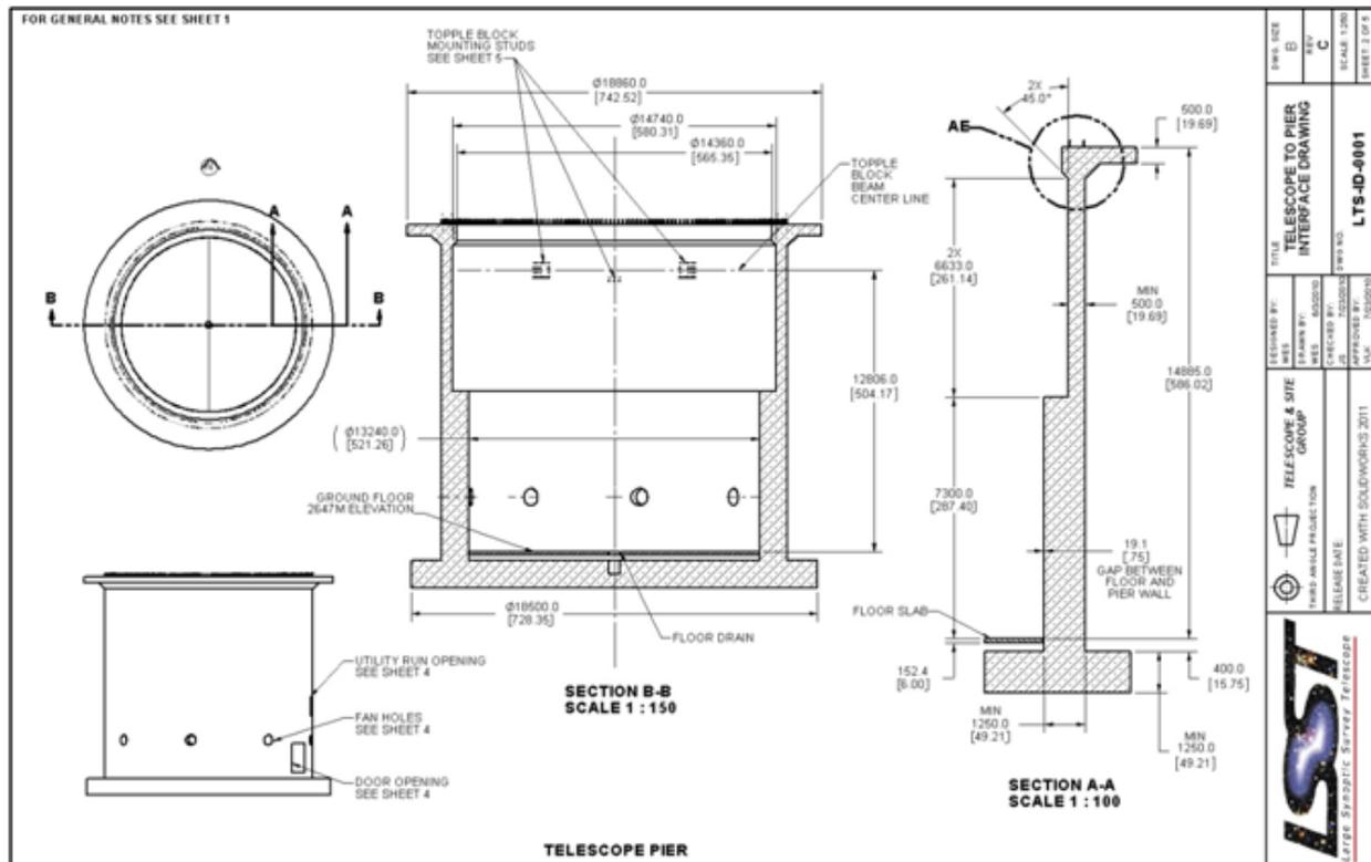
Figure 2.1-2: LSST Telescope Mount Assembly to Pier ICD.
