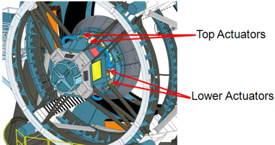
Figure 7.2.2-1: M2 Hexapod Actuator to Spider Spindle Attachment Locations
