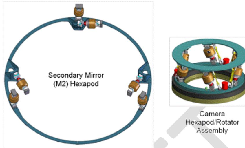
Figure 1.3-7: LSST M2 Hexapod and Camera Hexapod/Rotator Assembly
