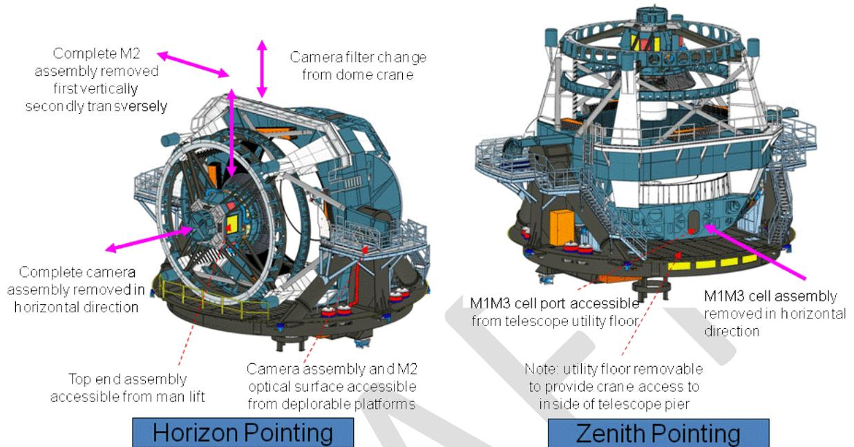
Figure 1.2-3. TMA Designed to Facilitate Maintenance.
