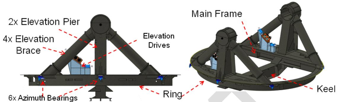
Figure 2.2.2-1. Azimuth Assembly Structure With azimuth bearings and elevation drives.
