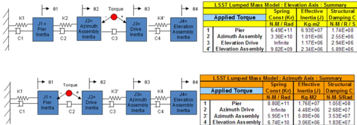
Figure 3.3-1: Lumped Mass Model of Telescope.
