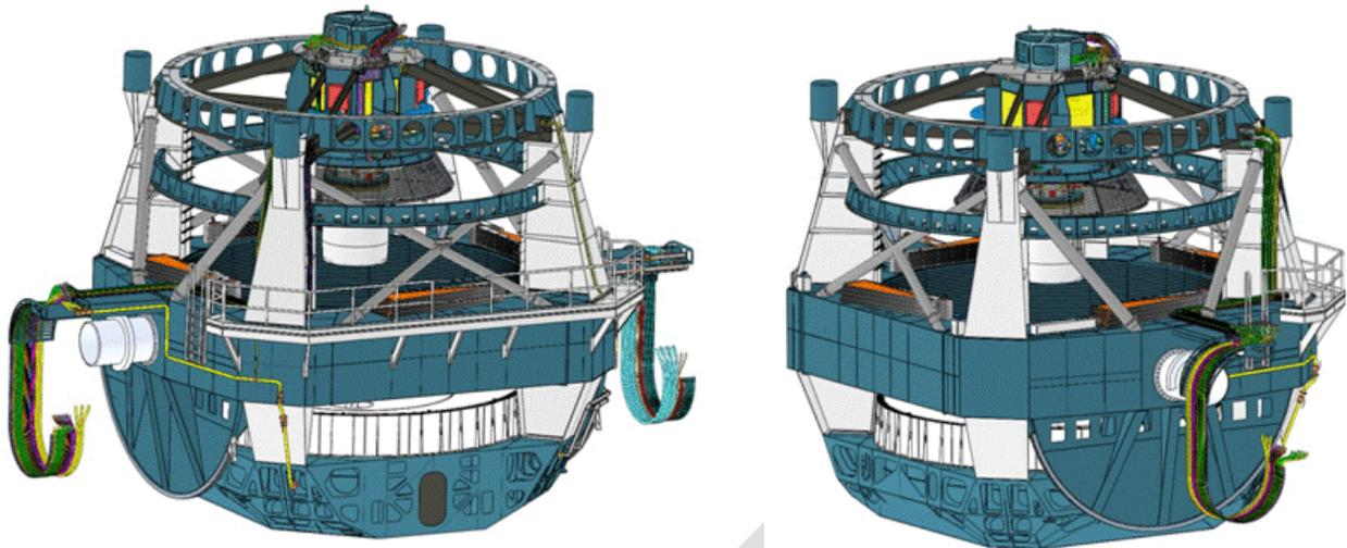
Figure 2.2.1-1. Elevation Assembly (with Cabling)
