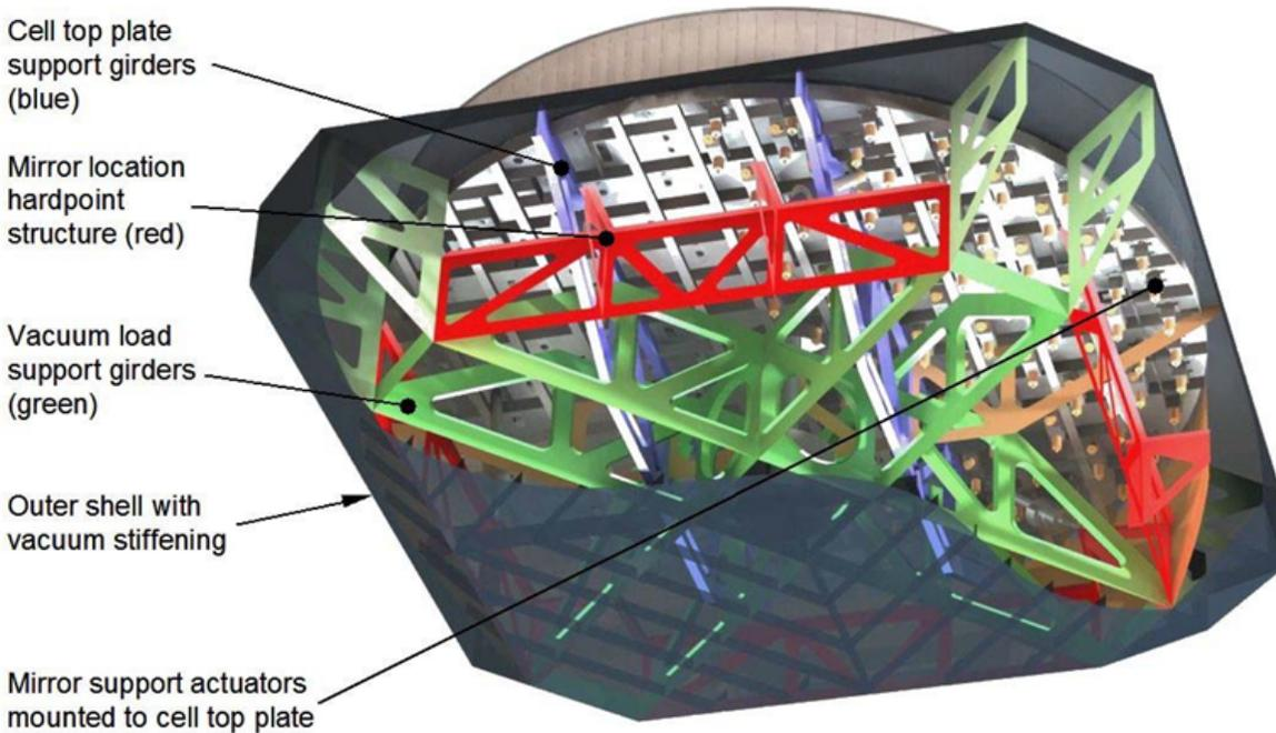
Fig. 7.1-2. Primary Tertiary (M1M3) Mirror Cell Assembly Structure
