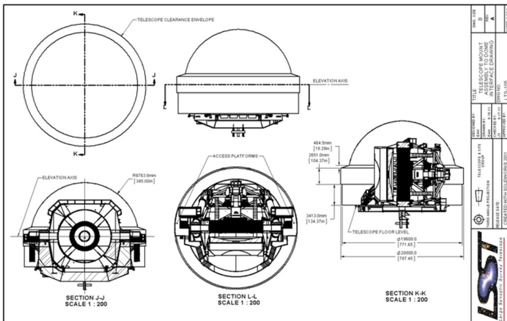
Figure 2.1-1: LSST Telescope Mount Assembly (with payloads) Design Envelope.
