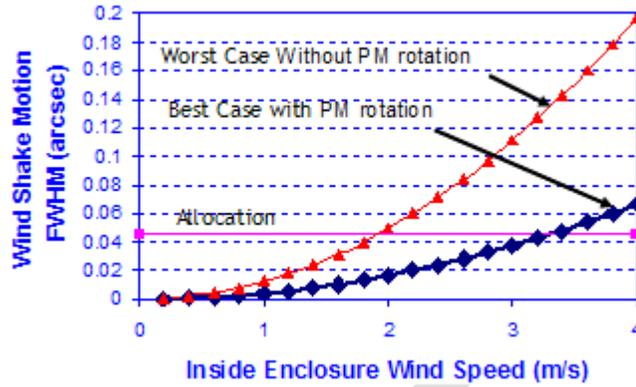
Figure 3.5-1: Pointing error as a function of internal wind speed.
