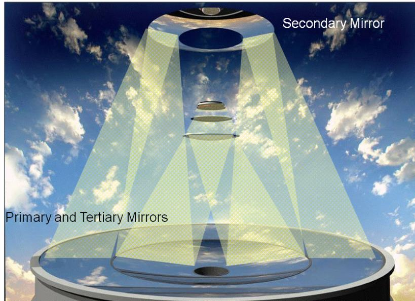
Figure 1.3-1 LSST Optical System.
