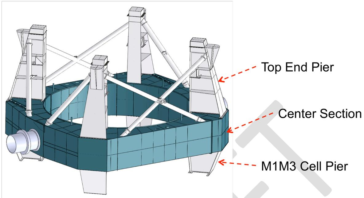
Figure 2.2.1-3. Elevation Assembly Center Section with Piers.
