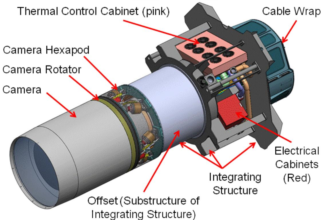
Figure 4.1-1: Camera Support Assembly
