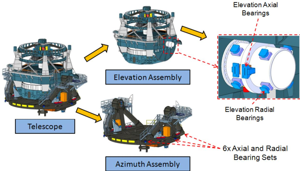
Fig. 2.3-3. Hydrostatic bearing configuration and locations on the TMA
