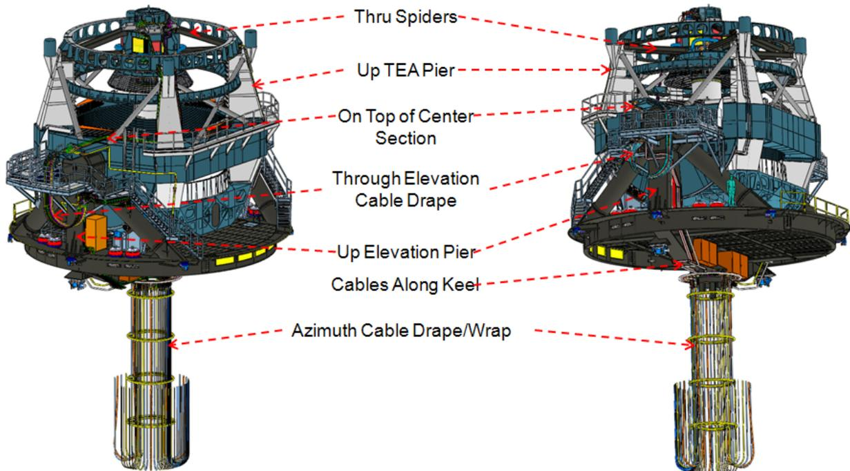
Fig. 2.6.4-1. Cable Routing.
