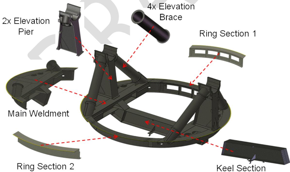
Figure 2.2.3-3. Main Structural Components of Azimuth Assembly.
