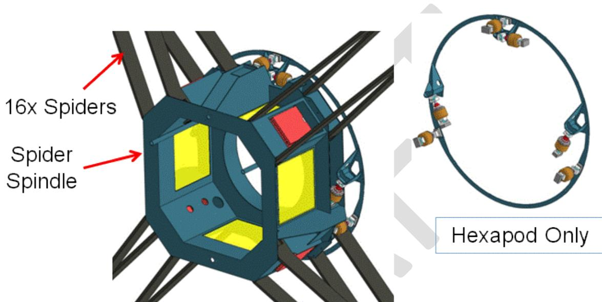
Figure 4.2.2-1: M2 hexapod installed on Spider Spindle.
