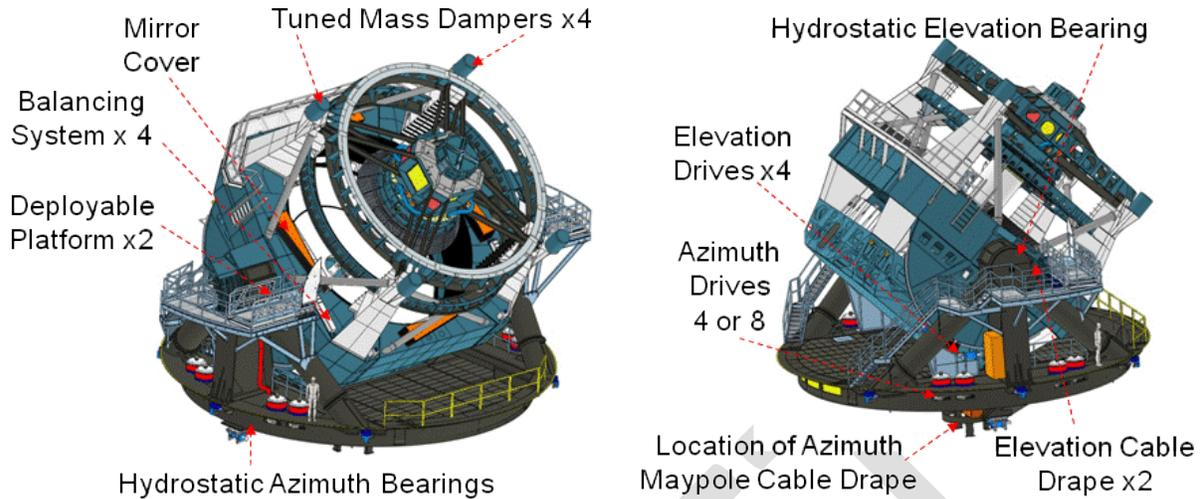
Figure 2-1: LSST Telescope Mount Assembly Overview.
