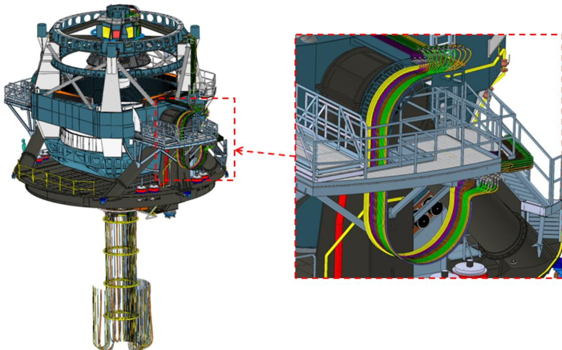
Fig. 2.6.2-1. Elevation Cable Drape
