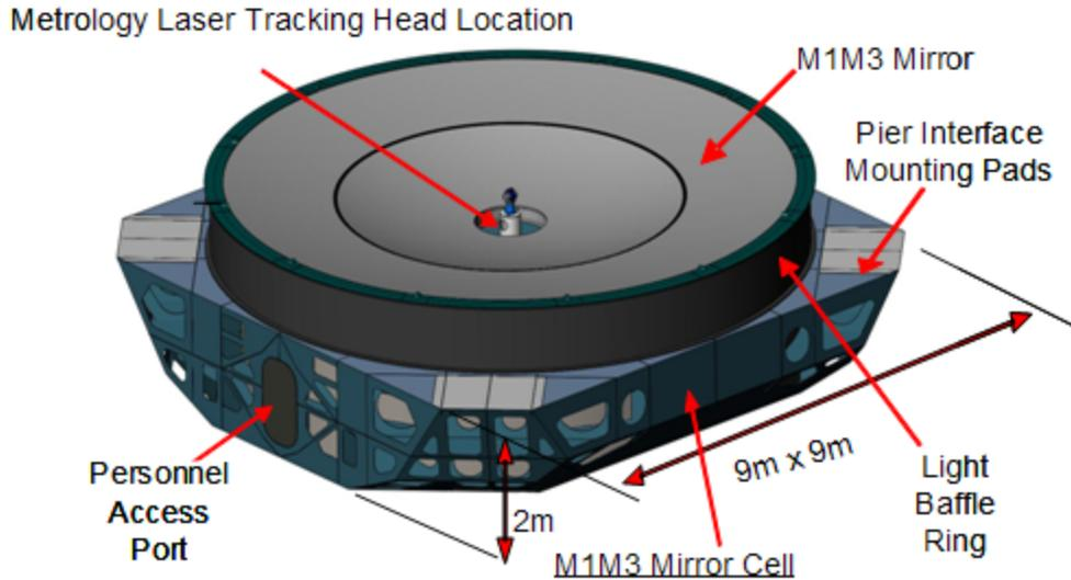
Fig. 7.1-1. Primary Tertiary (M1M3) Mirror Cell Assembly.
