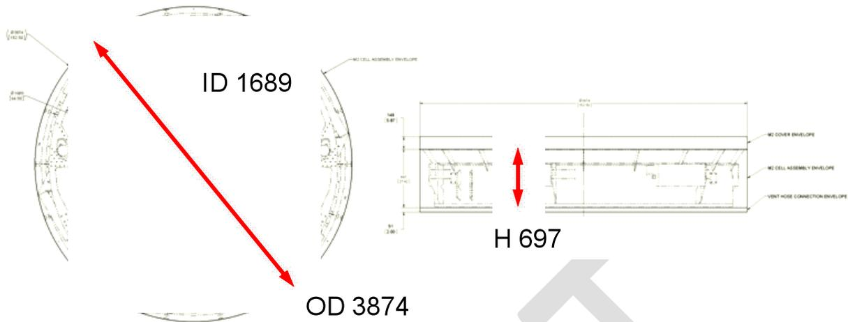
Figure 7.2.1.2-1: Simplified Design Envelope in millimeters.
