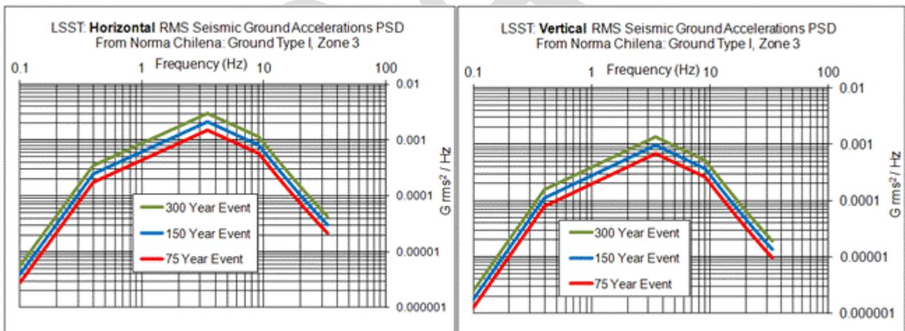
Figure 3.7-2: Seismic Ground PSDs determined from Chilean Building Codes.
