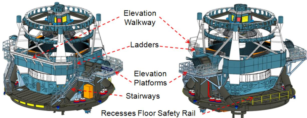
Fig.2.12.2-1 TMA Platforms, Stairways, Ladders and Safety Rails.
