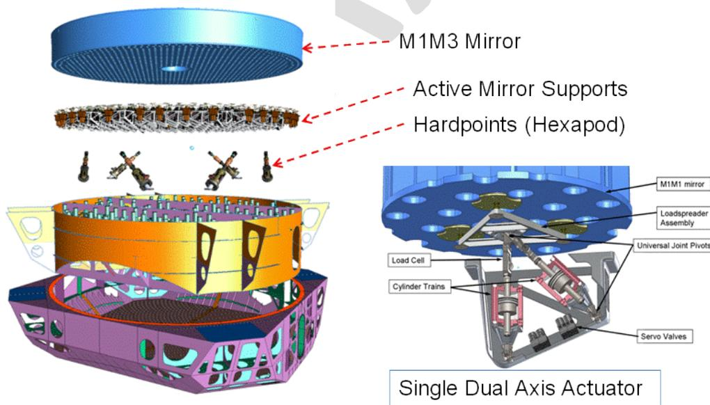
Figure 1.3-2. Primary/Tertiary (M1M3) mirror and support systems.
