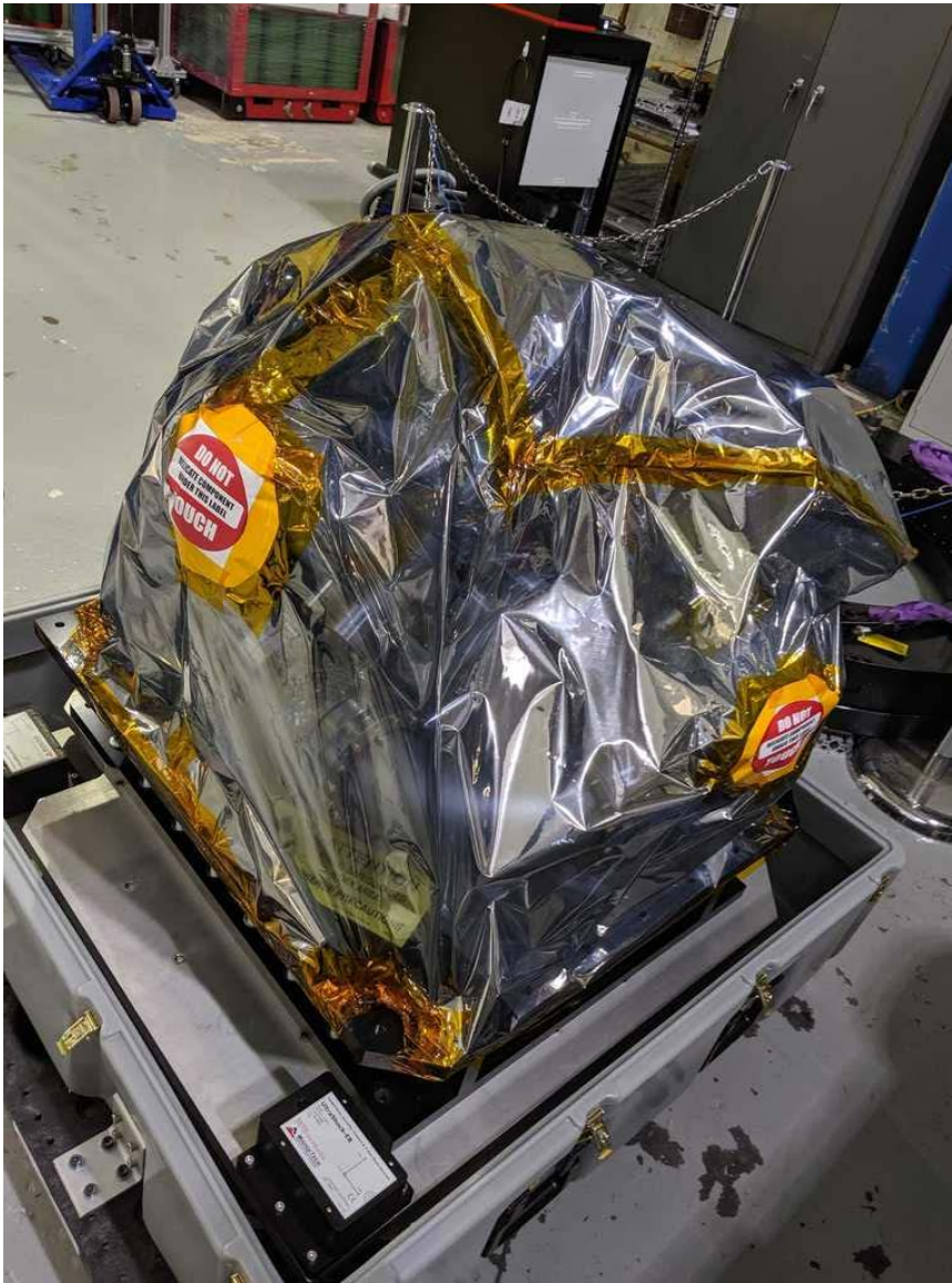
Figure 14: A view of the ComCam dewar outside the IR2 main area during packaging for shipment to Tucson. The two small black boxes attached to the base of the shipping container contain sensors to record conditions inside the container during shipment.
