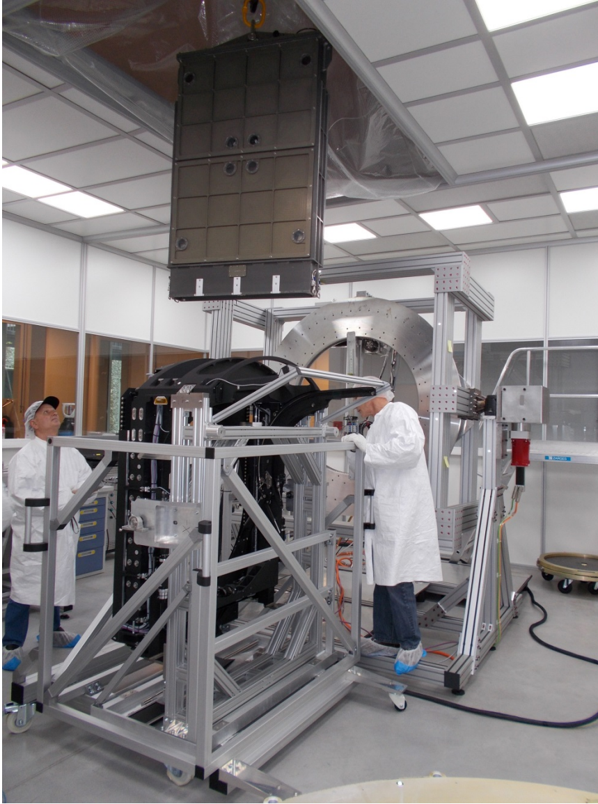
Figure 4: Preparations are underway for combined testing of the first units of the auto-changer and filter loader at the LPNHE cleanroom. Here the auto-changer is attached to its standalone test bench with the loader suspended overhead. Behind the auto-changer is the full-scale filter-exchange test bench that will be used for combined testing. The full-scale bench allows interoperation of filter-exchange components in all expected Camera orientations.
