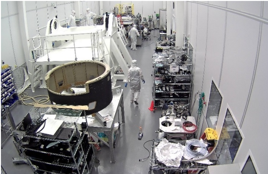
Figure 11: A view of the high-bay area at IR2 that shows the Camera integration stand with platform installed. The technicians in the view show the scale of the integration stand, which is the largest structure that will occupy IR2. The I&T team will use several other fixtures not shown to construct or store Camera subassemblies during the Camera integration process.
