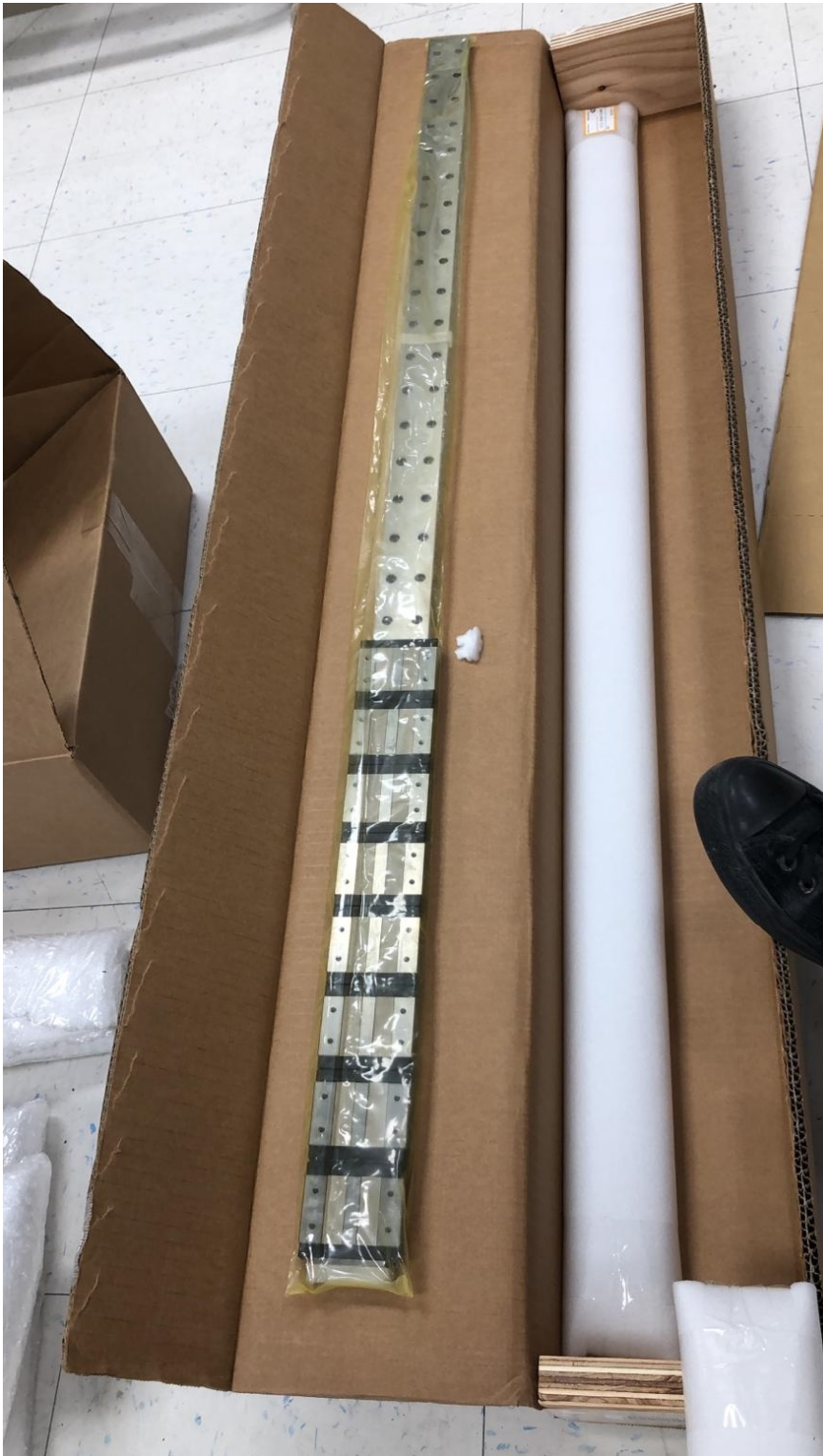
Figure 6: The drive-side linear guide assembly for the production shutter was delivered by the vendor to SLAC in early June. The guide carriages (eight square structures in the lower-half of photo) attach to shutter blade stacks and shutter-drive belts. The belts pull the carriages over the guide to open and close shutter blades.
