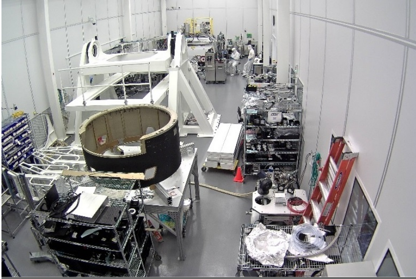
Figure 10: A view of the high-bay area at IR2 from a camera that faces the south side. In the foreground is the Camera body housing on an assembly bench. The housing is a protective structure that will enclose the cryostat assembly, L3 lens, Camera shutter, and filter-exchange components. The large white structure directly beyond the housing is the Camera integration stand, which will cradle the Camera assembly during construction. In this view, the platform of the stand is not installed yet and sits on the floor to the right of the stand. At the back of the room, technicians work in the BOT area.
