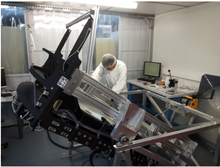
Figure 6: At CPPM, testing for the first unit auto-changer on its standalone test bench. Here the auto-changer is oriented at 45 degrees to the horizontal. On the Camera, the auto-changer can be used to swap a filter from online position in front of the L3 lens to one of the five storage positions on the filter carousel.
