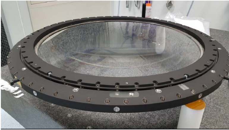
Figure 5: Early stages of integration of the L3 lens with its barrel. Here, the front side of the barrel is shown. The barrel is also called the cryostat front flange.
