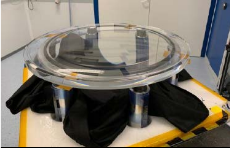
Figure 3: REOSC successively completed Broadband Anti-Reflective (BBAR) coating of the L3 lens and returned L3 to Thales SESO (TSESO) for inspection. The Optics team determined the lens meets project requirements.
