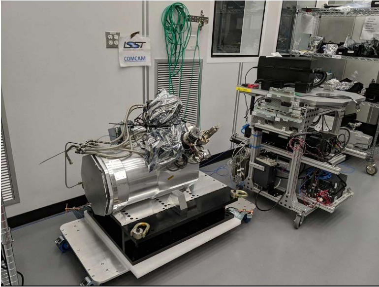
Figure 1: ComCam Dewar mounted to its stage plate at the SLAC IR2 Cleanroom Facility.
