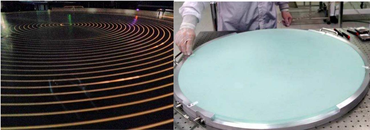
**Figure 2 Prototype Flat Field Screen using a leaky fiber placed in a spiral groove, plus optical diffuser.**
