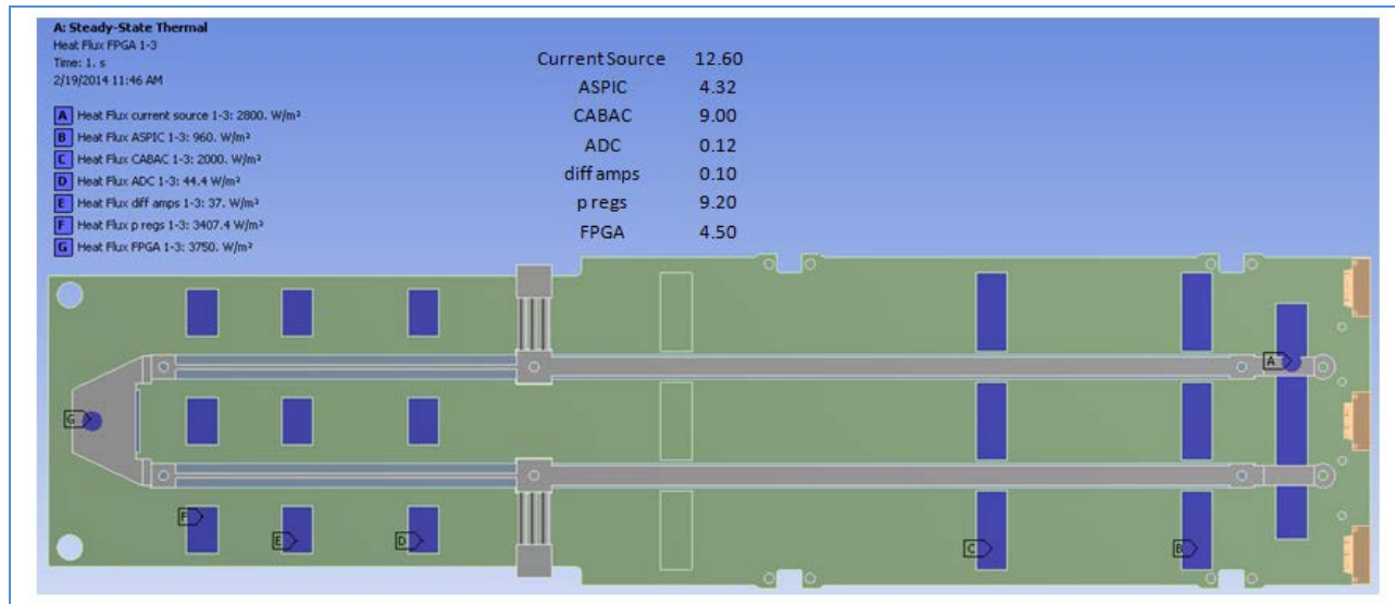
Figure 10-13: Thermal model, REB inputs
