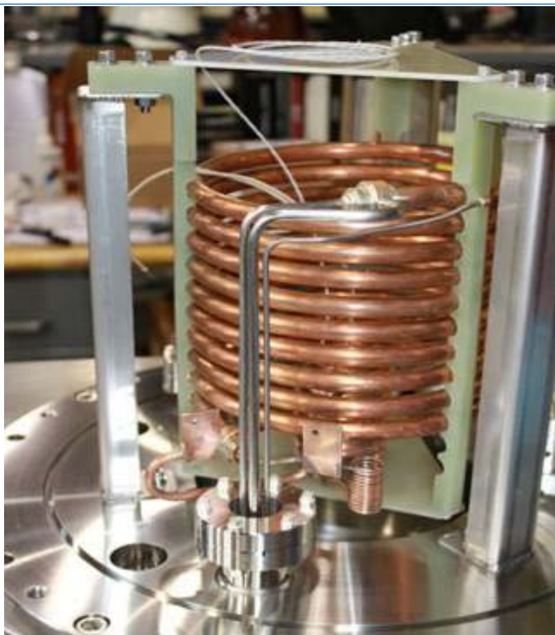
Figure 12-43: Prototype of counterflow heat exchanger, exchanger is constructed of 13mm (1/2 inch) OD copper tubing making the outer jacket, coiled to a 200mm diameter X 300 mm tall package.
