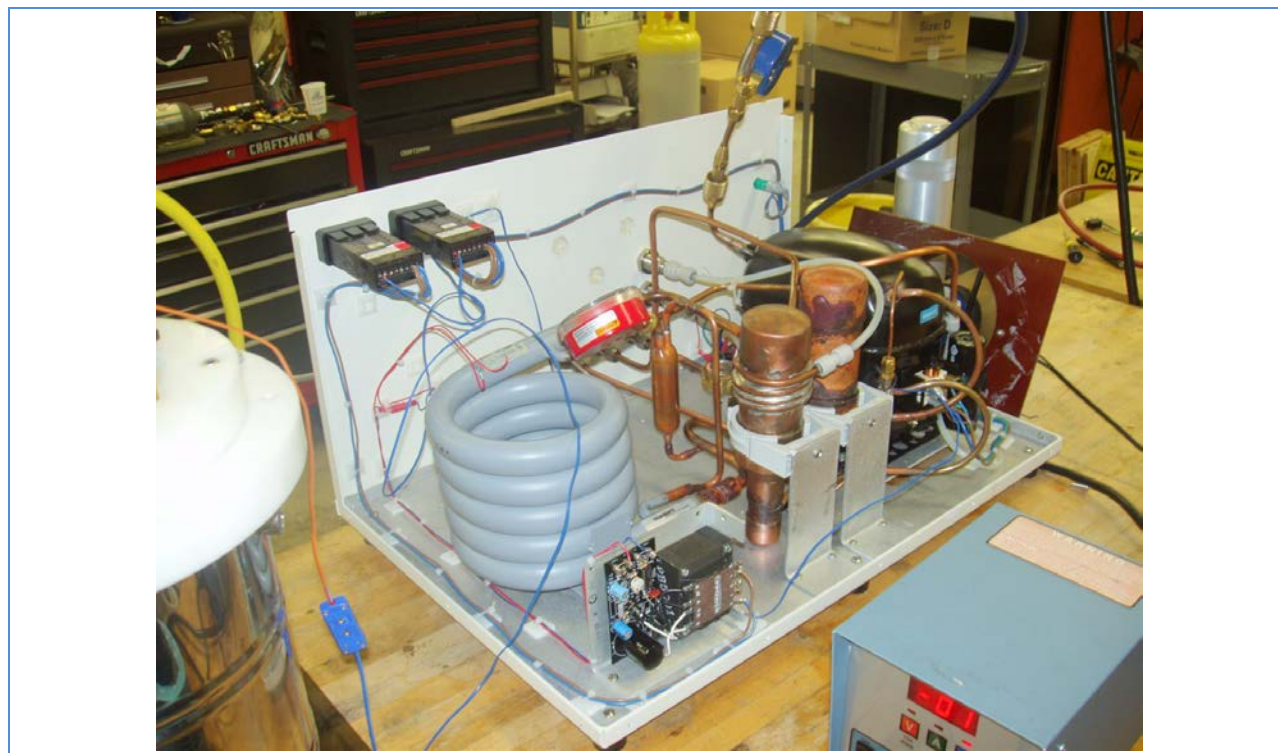
Figure 12-41: Prototype chassis holding compressor, oil separator, fractionating column at MMR lab
