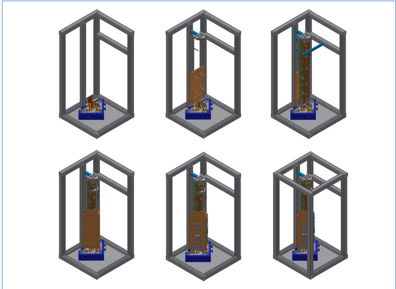
Figure 11-16: Corner raft tower assembly sequence
