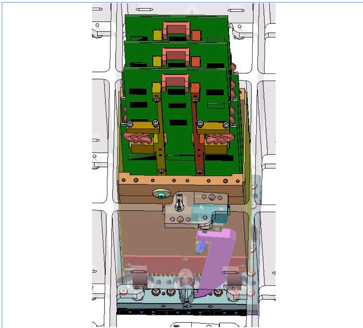
Figure 12-10: Hold down features at the base of the grid
