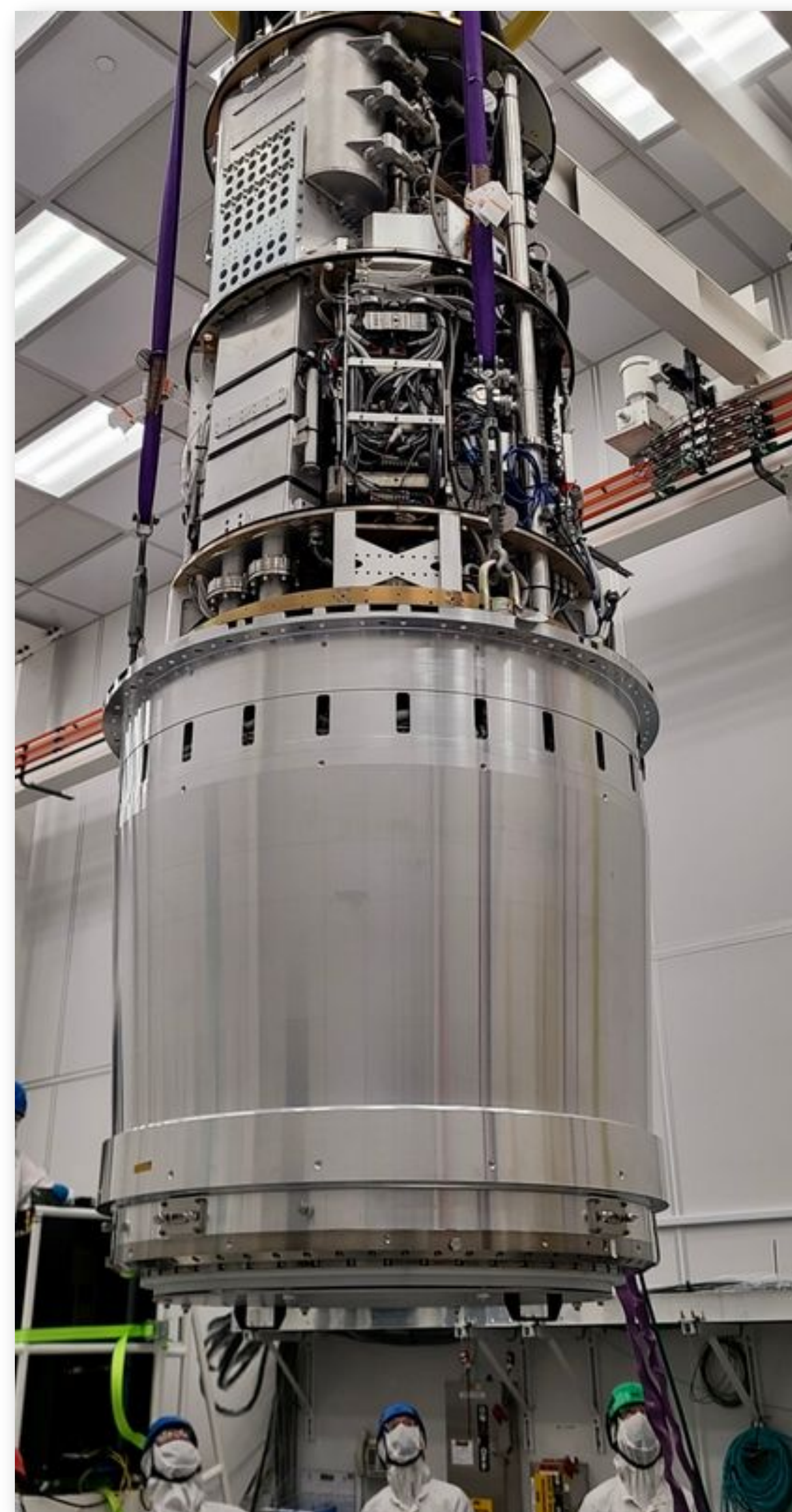
Cryostat and Utility trunk mated
