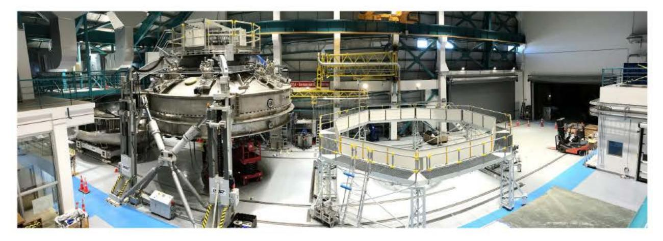
In July, 2019, Rubin Observatory's coating chamber was used to coat the glass Secondary Mirror (M2) with protected silver. It will coat the Primary/Tertiary Mirror (M1M3) with aluminum.
