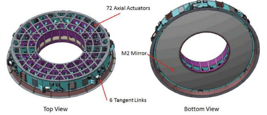
At 3.42 meters in diameter, the Rubin Observatory secondary mirror (M2) is the largest convex mirror ever made. The mirror blank is composed of an ultra-low expansion glass (ULE) from Corning USA to form a 100mm-thick meniscus mirror.
